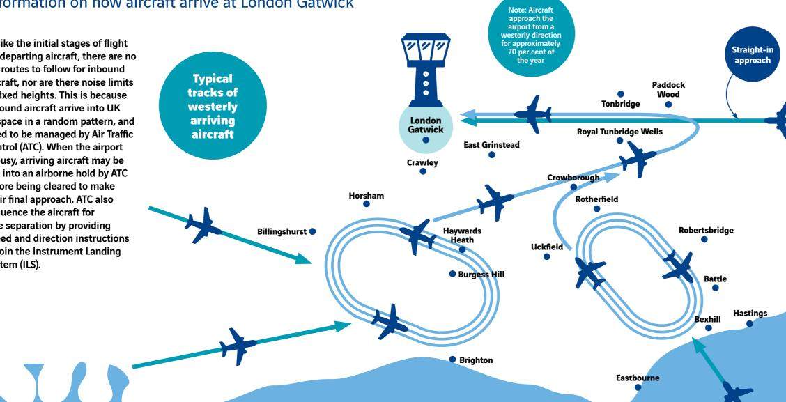
The ILS is a radio beam which extends out a horizontal distance of 25 nautical miles (nm) from the runway threshold and is aligned with the runway centreline to quide aircraft to land. Landing is a very busy and critical stage of the flight so it's vital that aircraft are set up for landing (with flaps correctly configured) and at the right speed some distance from
